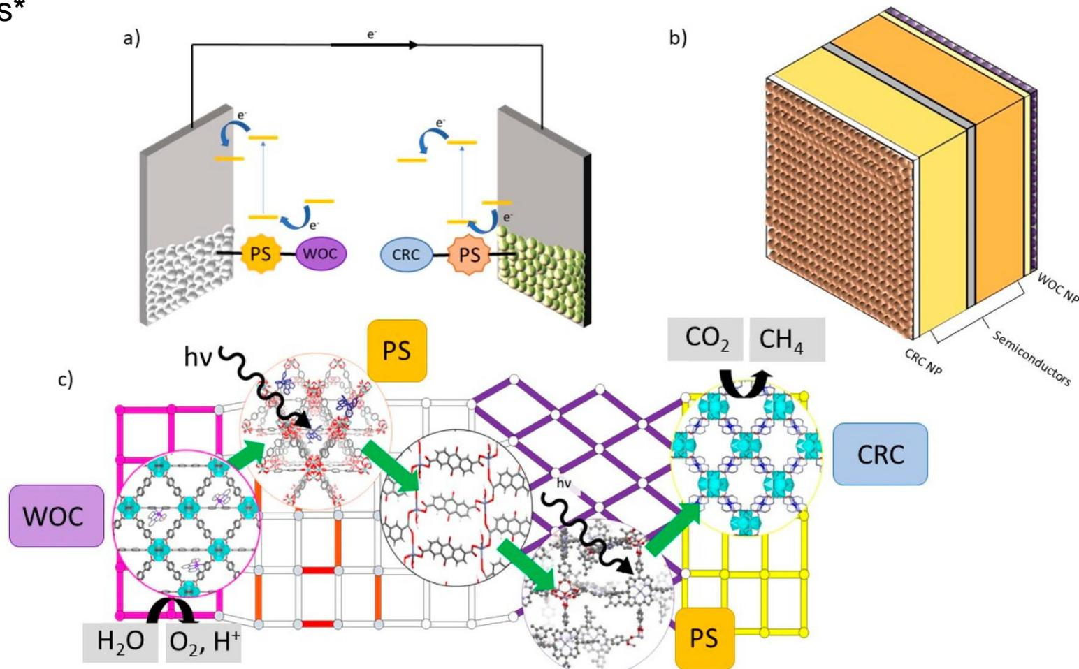
Schematics for artificial photosynthetic assemblies showing DSPECs featuring a photosensitizer (PS), water oxidation catalyst (WOC), and CO<sub>2</sub> reduction catalyst (CRC) (a), multijunction semiconductors with catalytic nanoparticles (NP) (b), and a proposed all-MOF artificial photosynthetic assembly (c).
