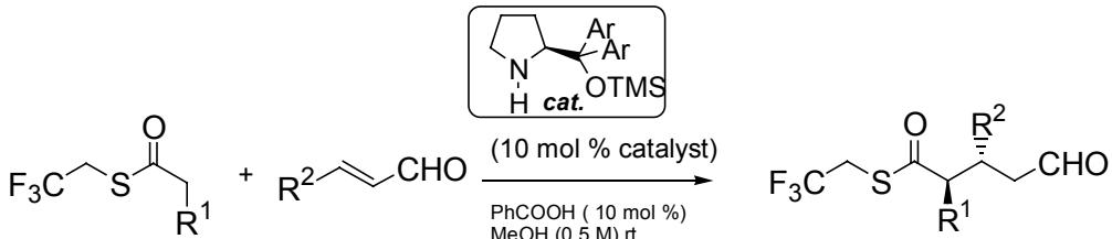
R<sup>1</sup> = Ph, X-C<sub>6</sub>H<sub>4</sub>, 1-naphthyl, 2-thienyl, PhCH=CH; 50-88 % yield, up to 86:14 anti/syn ratio, 66-98% e.e.
