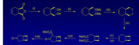
(i) LiAlH<sub>4</sub>, THF, Reflux (80%); (ii) MsCl, NEt<sub>3</sub>, DCM, -40 °C to RT (80%); (iii) Nal, Acetone, Reflux (70%); (iv) t-BuLi, Pentane-ether (3:2), -25 °C; (v) NalO<sub>4</sub>, RuCl<sub>3</sub>.H<sub>2</sub>O, MeCN, EtOAc, H<sub>2</sub>O; (vi) MeOH, Conc H<sub>2</sub>SO<sub>4</sub> (85% from di-iodide); (vii) KOt-Bu, THF, Reflux (95%); (viii) DMSO, H<sub>2</sub>O, 155 °C (97%).
