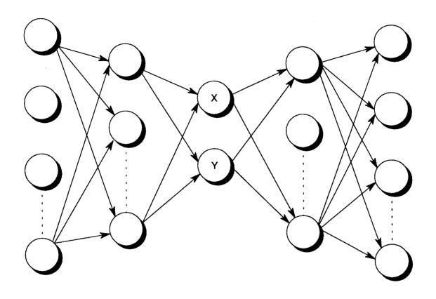
Input Layer Encoding Layer Parameter Layer Deconding Layer Output Layer
