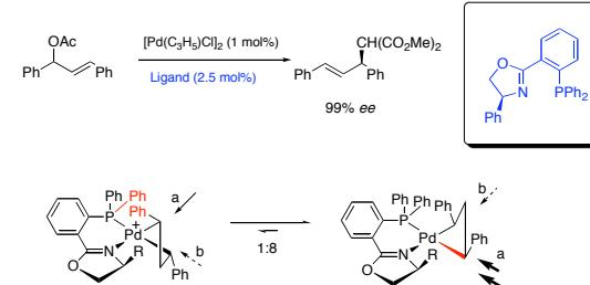
Attack via *a* is observed but stereoelectronics should favor attack via *b*
