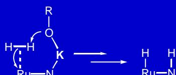
base-assisted heterolysis of hydrogen in the hydrogenation of ketones, as proposed by Chen
