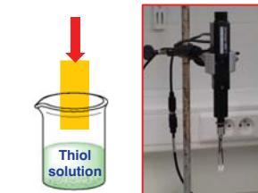
Schematic representation of the gradient generation through the action of a linear actuator
